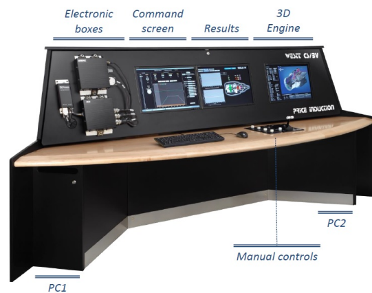
(b) Price Induction WESTT CS-BV: DGEN 380 turbofan engine virtual test bench (©Price Induction) [71]
